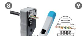
• Visually check that the wires are fully inserted, and the wires are not touching each other
